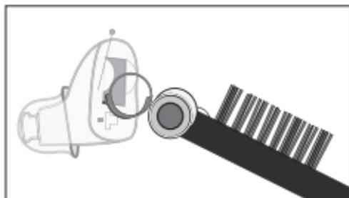
2. Insert the button cell battery (type PR70/ A10) included in the delivery into the battery compartment as shown. When inserting the battery, ensure that the correct polarity (+/-) is observed. The magnetic part of the cleaning brush makes this step easier for you. The hearing amplifier is switched on by closing the battery compartment.
