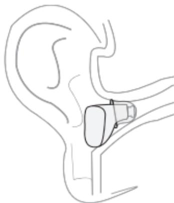
ing amplifier too deeply into the ear canal. If the earplug is not properly in place or feels uncomfortable, try a different earplug. If this also does not result in a much better fit for the hearing amplifier, you have the option of using each device in the other ear.
